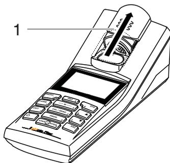
**Inserting a 28 mm cell**
