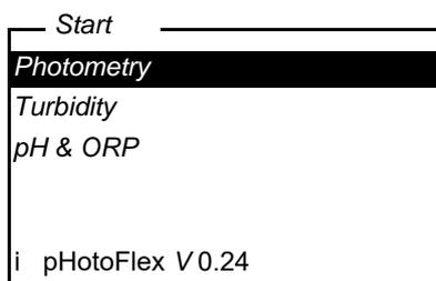
After a few seconds, the meter automatically switches to the measuring mode and measured parameter used last.
